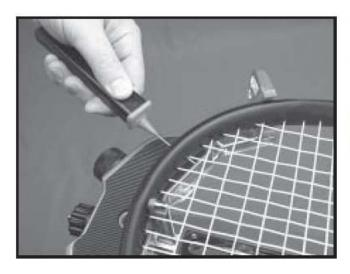
The machine includes the Pathfinder stringing awl which creates a pathway between or around strings to make inserting a string through tight grommets easier and quicker.
