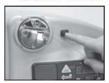
To tension a string, push the tension switch or the foot pedal. The string gripper will rotate and slowly apply tension to the string. When the set tension has been attained, the gripper will stop rotating. As the tensioned string stretches, the gripper may rotate intermittently, maintaining the set tension.
