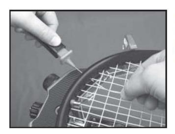
Once the awl is inserted, pull the handle of the awl outward while holding the tip section in place, leaving the outer sheath in the grommet hole.
