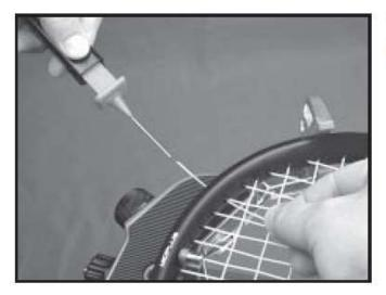
While holding pressure on the string, slowly pull the sheath out of the grommet hole to leave the end of the string exposed.
